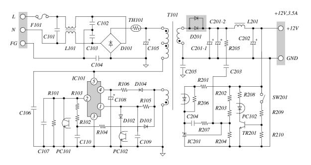
Fig.6 MR1520 Standard Power Supply Circuit 85V to 132V input, 12V, 3.5A output
