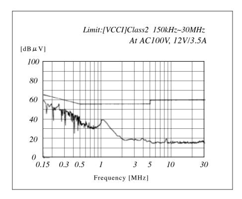
Fig.10 Input Feedback Noise
