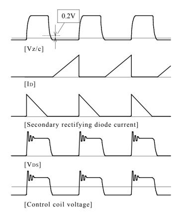
Fig. 1 ON Trigger Operation Sequence
