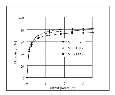
Fig.8 Efficiency Characteristics (standby)
