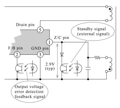
Fig.2 Standby Mode Selector Circuit
